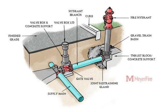
Here, the connection to the water source is at the "Joint-retraining gland" right around where the pipe goes vertical at the 90-degree bend. After that point, the hydrant is dry. So that's the spot where there's a connection to the main water source and where City maintains responsibility for repair and maintenance. Staff in Fire and Municipal Utilities tell me this has been the standard practice and is exactly how the sentence in the 2018 letter reads.
